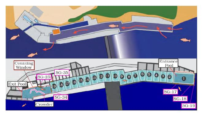
Figure 1. General overview of Tumwater Dam (top), and specific pool and gate configuration. Fishway PIT-arrays are located at Weir 15 (downstream) and Weir 18 (upstream). The fishway was designed to have SG-34 open and SG-35 closed for normal passage, and the opposite configuration for trapping activities.
