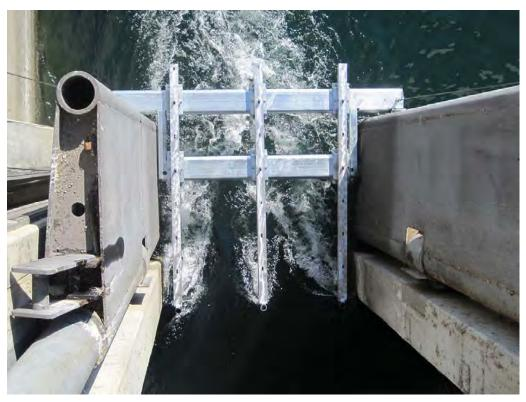
Photo 3: Looking down on the ADV trolley shown inserted in the bulkhead gate slots. (This photo was taken by Jacobs Engineering during the trolley testing in Feb 2011)
