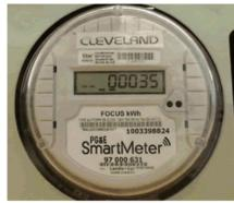
therefore need to be billed for. The newer meters are able to gather more information about electricity usage, not just overall usage. They can measure when you are using electricity throughout the day, for example. They can also communicate this information to the power company wirelessly, eliminating the need to have someone come to your home to read the meter.
