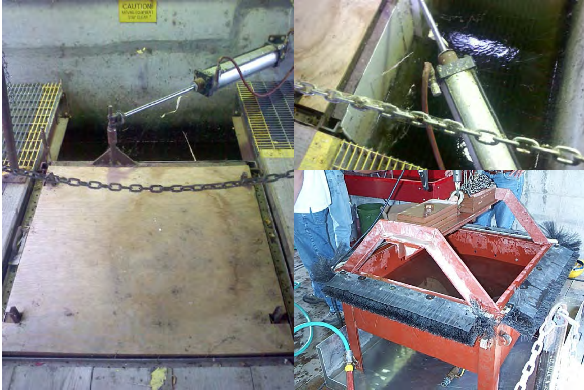
Figure 1. Adult trapping facility at Rocky Reach Dam. The pneumatic arm (left and top right) activates a gate that guides fish into a holding vessel (bottom right, shown lifted). Trapped fish are either allowed to exit the holding vessel by opening the gate, or are lifted for processing.
