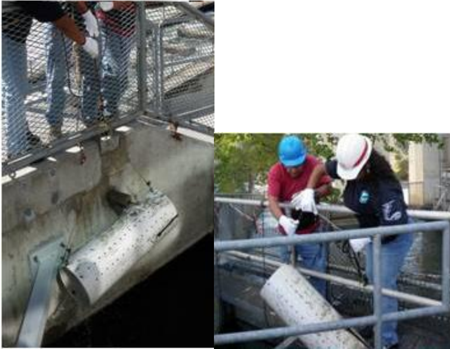
Figure 3. Examples of tube traps used in Lower Columbia River dams for adult Pacific Lamprey collection.
