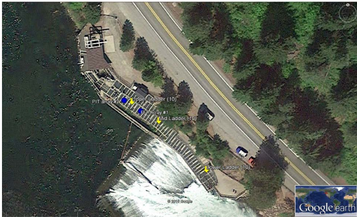
Map 1. Close-up of Tumwater Dam Fish Ladder proposed release locations (yellow arrows; 10 adults in each release, 30 total). Lower ladder release will be in slot #1, mid ladder release will be in slot #12, and upper ladder release will be in slot #17. Of the total 19 slots within the ladder, the two PIT tag arrays (blue circles) are located in slot #15 and #18 of the fish ladder. See Addendum for more details.
