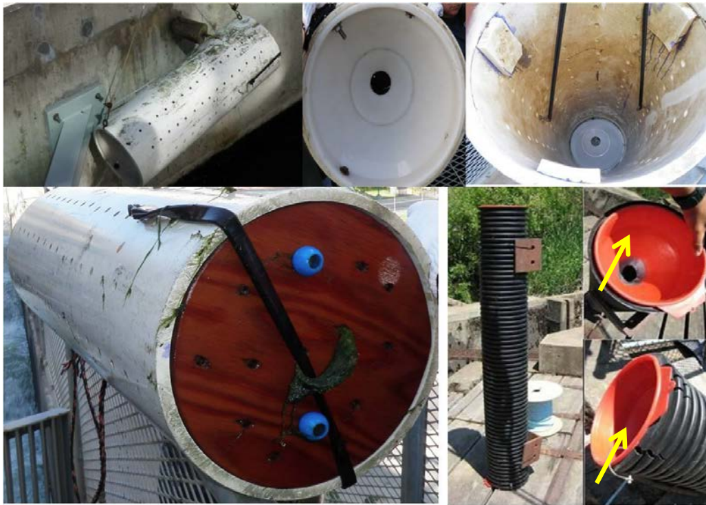
Figure 2. Examples of tube traps proposed to be used for lowering adult Pacific Lamprey in Tumwater Dam fish ladder. Yellow arrows indicate the area where a separate rope will be attached to detach the funnel on one side from the tube trap.
