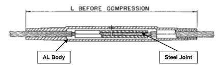
Application: Used to splice ACSR overhead conductor in full tension.
